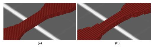
**Figure 2.** The difference between the extruded lines of (**a**) 0.4 mm nozzle diameter and (**b**) 0.8 mm nozzle diameter.
