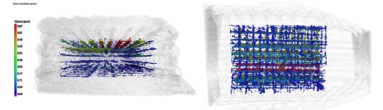
Figure 8. CT image of the porosity system of a 3D-printed sample.
