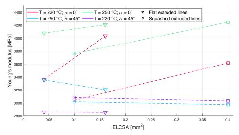
**Figure 11.** The change in Young's modulus based on different parameters: on the left side, the two nozzle diameters used with a flat extruded line and, on the right side, the two nozzle diameters used with the more circular extruded line can be seen linked together.
