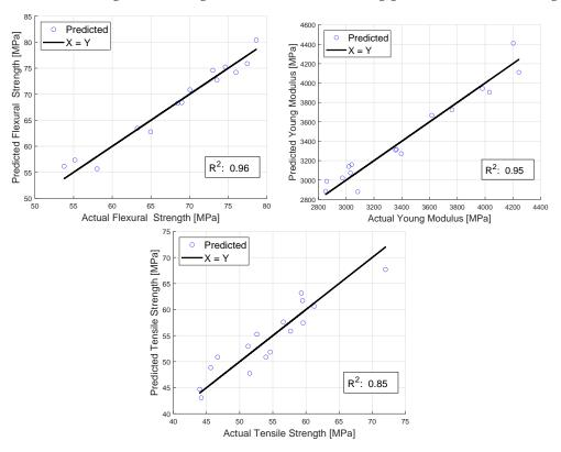
Figure 13. Performance of the model used for all three mechanical properties studied.
