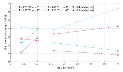
Figure 9. The change in tensile strength based on different parameters.
