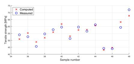
Figure A2. Comparison of the computed and the measured tensile strength.
