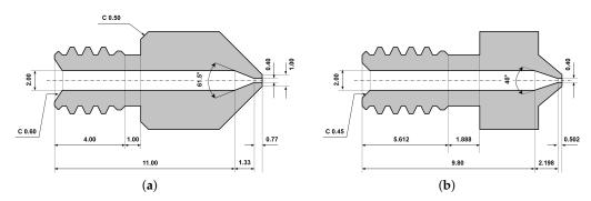
Figure 5. The difference between the (a) MK8 nozzle and (b) V6 nozzle.
