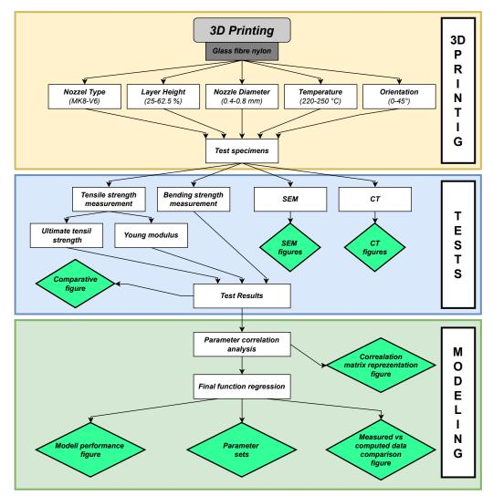
Figure 1. Summarization of the tests and methods used during the research phase.
