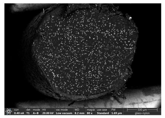
Figure 6. SEM image of the distribution of the chopped glass fibres inside the filament.
