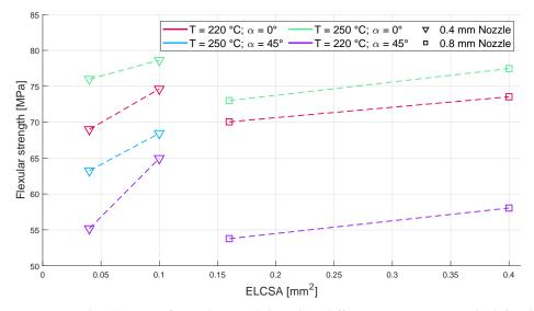
**Figure 10.** The change in flexural strength based on different parameters: on the left side, the two layer height used with the 0.4 mm diameter nozzle and, on the right side, the two layer height used with the 0.8 mm diameter nozzle can be seen linked together.
