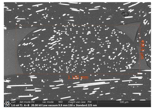
Figure 4. SEM image of ELCSA inside a 3D-printed layer.
