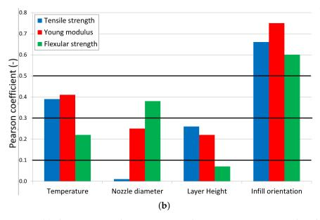
**Figure 12.** (**a**) The Pearson correlation matrix regarding printing parameters and mechanical properties of samples and (**b**) the summarization of the Pearson coefficient values of the same matrix.
