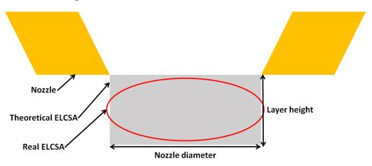
Figure 3. The correlation between nozzle diameter, layer height, and real and theoretical ELCSA.
