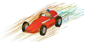
Wind tunnel simulation with translating wall
